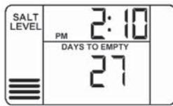
**NOTE:** For the first several weeks of operation the **DAYS TO EMPTY** may provide erratic operation. For example, the blue indicator light may flash, showing that more salt is required when the actual salt level in the tank is well above the Level 0. In some cases, the **DAYS TO EMPTY** may even increase over a several week period.
